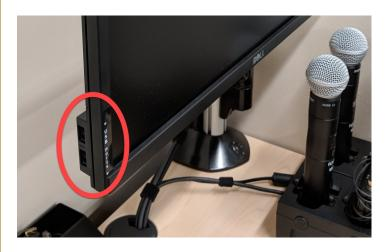
The podium computer's USB Ports for flash drive or clickers are located on the bottom left side of the monitor.
