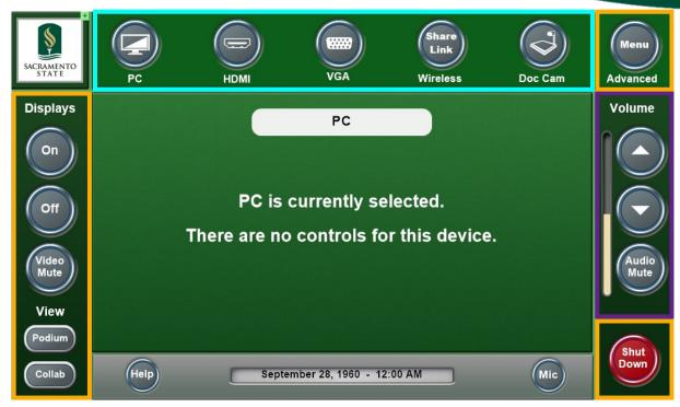
Display Controls on left and right (yellow box). Sources on top (blue box). Audio Controls on the right (purple box).
